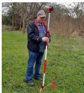
Ron Davis holding the ranging rod while setting up the TDS. (photo by John Rich)
