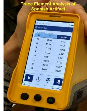
Measuring Spanish lead ball prior to XRF testing
