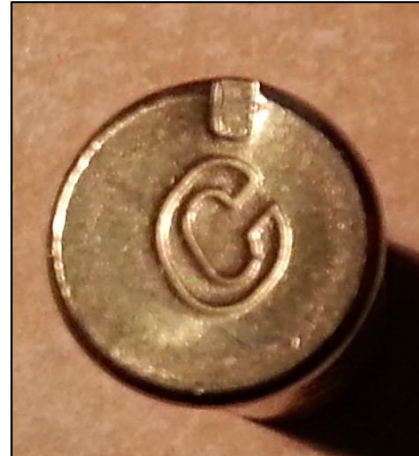
Figure 2. Firing pin imprint on the base of a .22 caliber rimfire cartridge. RIMFIRECENTRAL.COM.
