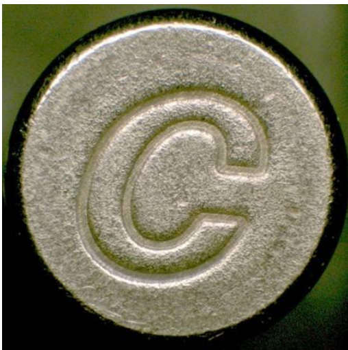
Figure 2. Headstamp on the base of a .22 caliber rimfire cartridge manufacture by Cascade Cartridge, Inc., of Lewiston, ID. Rimfire Headstamps
