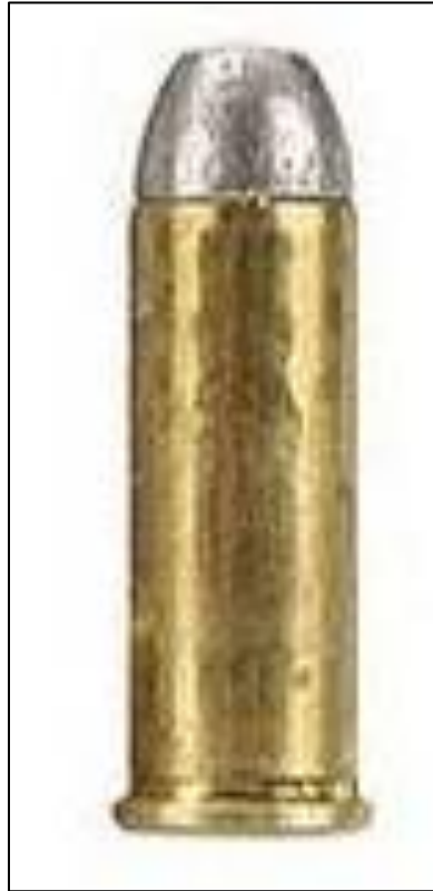
Figure 3. A centerfire, brass cased, .38 caliber, Long Colt, revolver cartridge, containing a lead bullet. This is a pristine version of the cartridge depicted in Figure 2, Picture from https://military-history.fandom.com/wiki/.38_Long_Colt_
